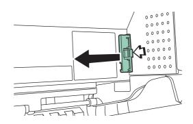
**4** Clean the filters using a vacuum cleaner or a dry cloth.
